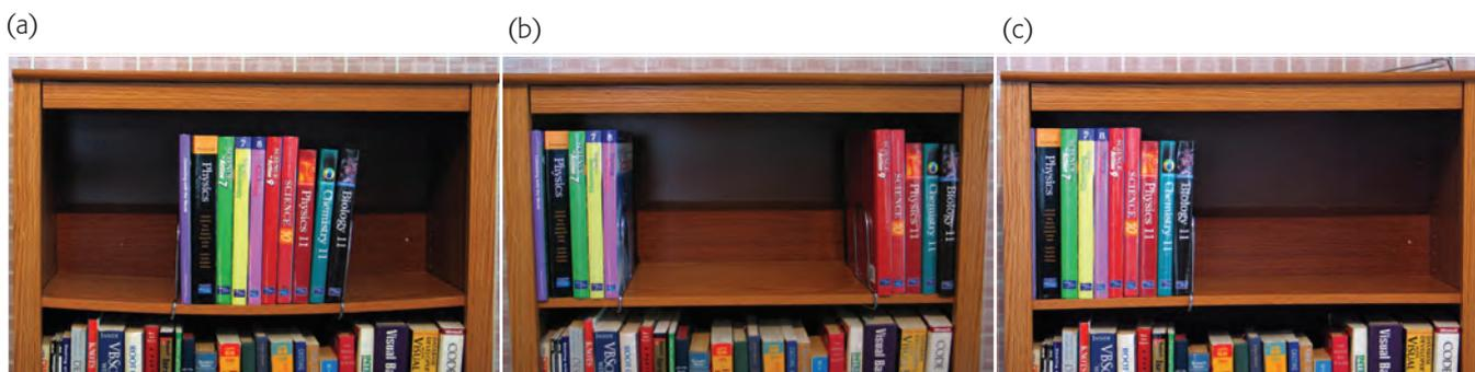
**Figure 4.19** When the books are placed in the middle of the shelf (a), the shelf may sag from the unsupported dynamic load. If you place the books nearer the supports ((b) and (c)), the shelf does not sag.
