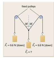
The above diagram shows a possible setup for a vertical force board. (You may prefer to modify the setup, however, using a force table instead of a force board, as suggested for this activity.) In this vertical force board, there are three different forces, each acting on a different string. If two of the forces are known, the third force can be determined. Describe how you would determine the unknown force  $\vec{F}_2$ .
