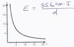
4. When a mass is placed on the free end of a board, the end is deflected downwards. The following table shows the downward deflection (d) corresponding to various lengths of board, as measured in each experiment. Each deflection was produced by the same mass.
