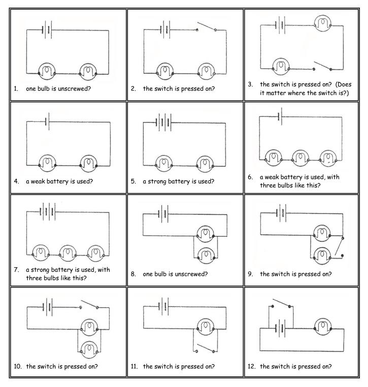
NOTE: Diagrams 11 & 12 are special situations. They are known as \_\_\_\_\_\_ circuits. Because there is no electrical load to use up the energy from the battery, the circuit heats up and may become hot enough to start a fire.
